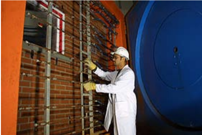
Dynamic wall testing facility for studying the effect of wind-driven rain on full-scale wall sections.
