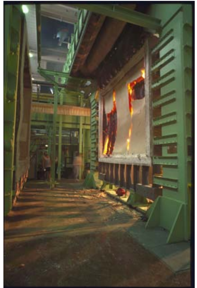
Full-scale experiment on the fire resistance of gypsum board.
